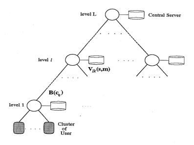
Figure 1: Logical network topology for VOD
